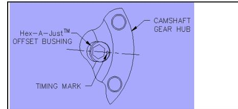
**Inserting Offset Bushing
