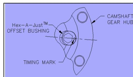
**Inserting Offset Bushing
