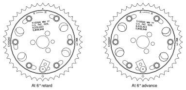
After the timing has been adjusted, remove the adjusting tool from the cam sprocket. Tighten the six bolts to 13-15 ft-lb.
