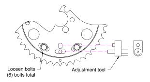
After the tool is inserted into the slots, use a 3/8 wrench to rotate the tool. There are seven timing marks indicated with an A and an R on the ends. Each timing mark is approximately 2° and is lined up with a single alignment mark on the outer camshaft sprocket member (Refer to illustration below).
